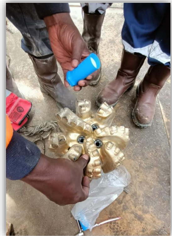
Preparation of PDC drill bit at a GDC rig at Paka Well
