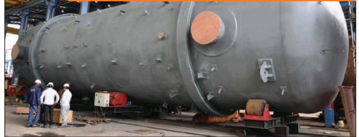
EWT Heavy Fabrication Yard Flare Knock-out Drum fabricated by EWT for EGINA FPSO project
